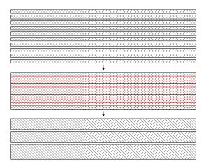
To produce multiple beams at once: leave away the glue
