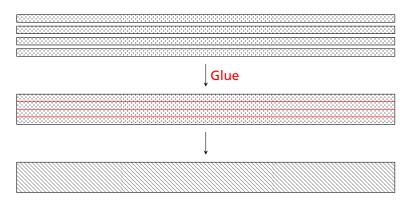
Wood slats are glued and pressed to beams.
